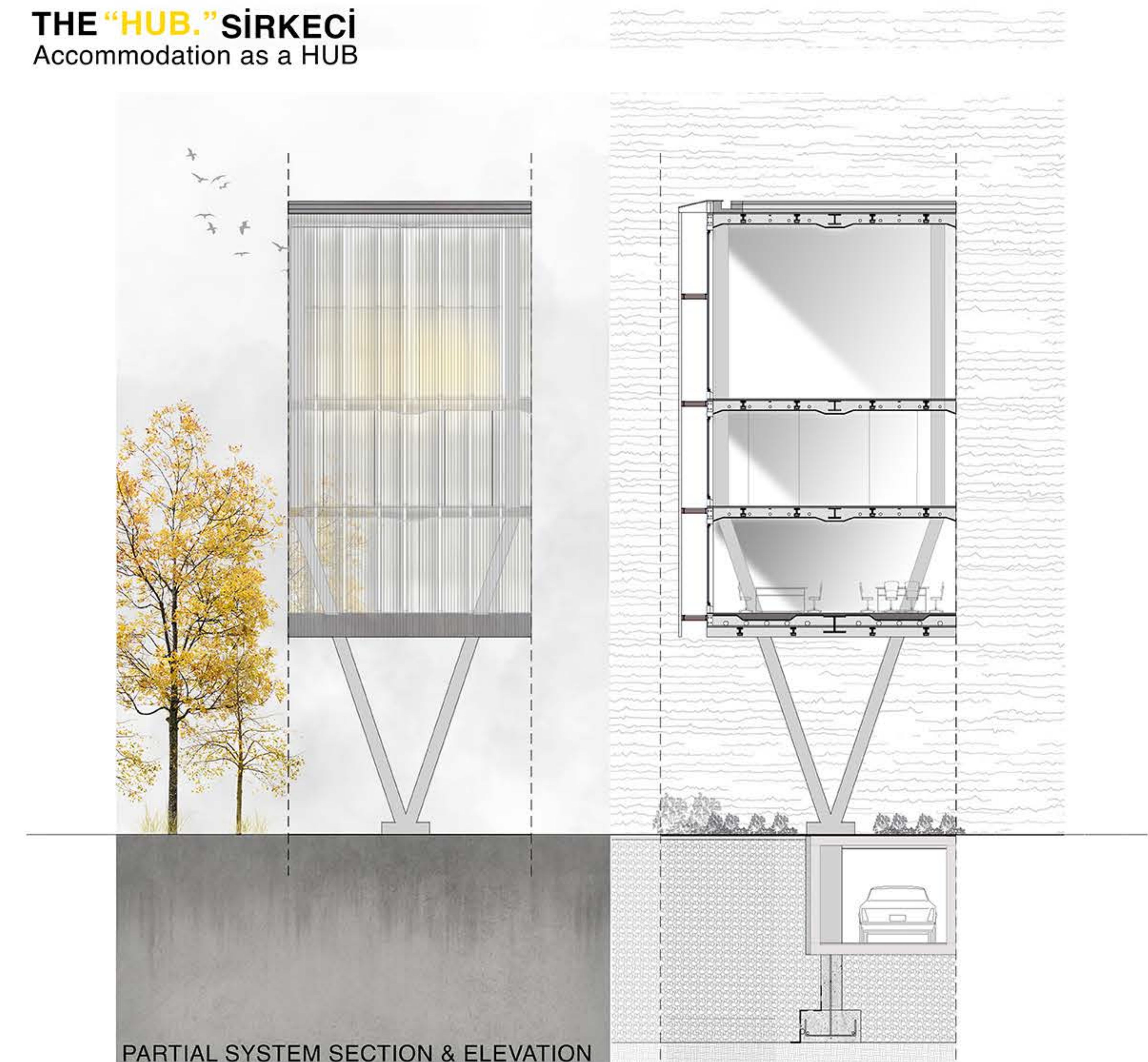
PARTIAL SYSTEM SECTION & ELEVATION
