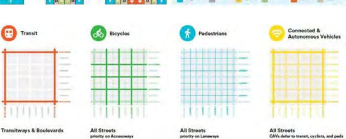
On Transitways, priority is given to transit vehicles — through designated lanes and signal priority — to travel at their desired speed. Bike-share and scootershare stations are co-located with transit stops to enable convenient transfers to other modes. Transit can also travel on Boulevards, but may not be given the highest priority. On Accessways, center-running bike lanes with green waves will allow comfortable cycling.
