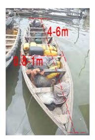
While designing the arteries, there were two main challenges; there should be enough space for canoe transportation and also to connect both sides of the axis, there needs to be some sort of a bridge. To have widths providing the needs for these within the narrow axes, the dimensions need to be precise and not wider than it should be.
