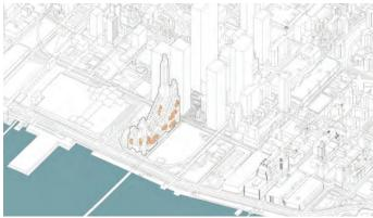
Various size voids are created on higher levels of the building, which acts as public spaces and terraces. These spaces are created for air ventilation and better use of sunlight. With these voids, the use of open-air spaces on high levels is eased.
