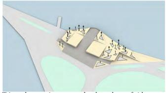
Triangular openings are made where the roof either tilts upwards or downwards in order to allow controlled sunlight into the building.
