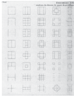
'Building Ensembles, Resulting from the Divisions of the Square, the Parallelogram and Their Combinations with the Circle', Jean-Nicolas-Louis Durand, 1802
