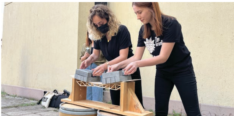
Pelin Halisipek, Beyza Keskin ve Sena Nur Yıldız testing their bridge. Load Carried: 28 kg, Bridge Weight: 126 gr, ARCH231, Spring'22.
